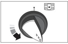
Adjust the flame height to suit by turning the knob. On this range the low position is beyond high, **not** between high and off. The 'LO' marks the low position. Turn the knob towards it after the contents of a pan have boiled.
